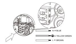
Connect AC wires correspondingly.
