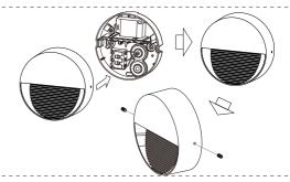
Fix the cover with side cap screws.
